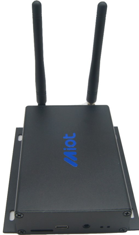
Picture 1.: Installation Connected with LTE FULL BAND Antenna *2 Available for LTE CAT4, CAT6 M.2 module Antenna Part Number: XXXXXX
